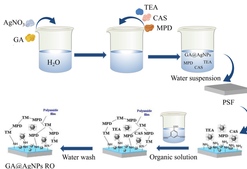
Figure 1: The process of preparation of the antibacterial RO membrane.
