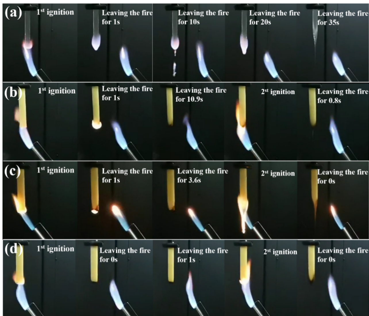
Figure 5: Results from UL-94 measurements for PLA/HCCP-EP blends: (a) PLA, (b) PLA/HCCP-EP-1, (c) PLA/HCCP-EP-3, and (d) PLA/HCCP-EP-5.
