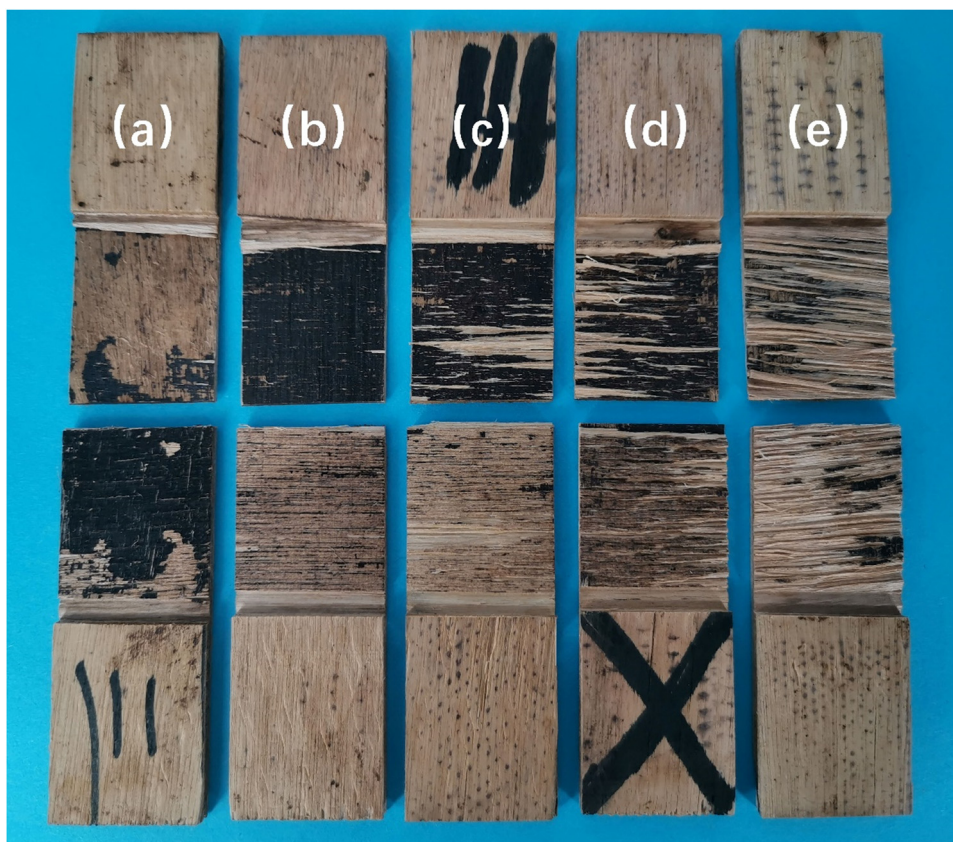
Figure 7: Influences of ECH on the wood failure of the wet plywood: (a) GKLE-10, (b) GKLE-20, (c) GKLE-30, (d) GKLE-40, and (e) GKLE-50.
