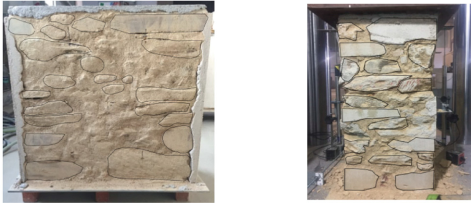
Figure 11: Specimens tested by direct and indirect sonic methods (Source: Van Eldere et al. [78]).
