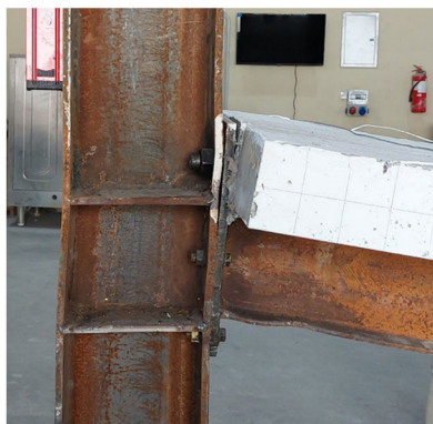
Figure 22: Failure of column in CM5.
