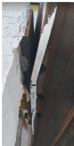
Figure 9: Failure of column flange in CM1.
