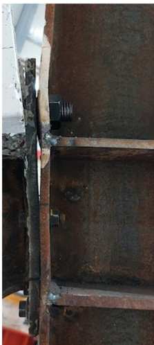
Figure 25: Shape of end plate welding with beam after test in CM5.
