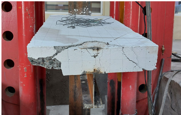
Figure 24: Shape of slab crashing in CM5.
