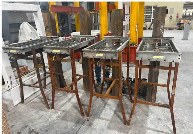
Figure 3: Preparing specimens for casting.
