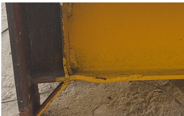
Figure 18: Shape of failure in beam of CM4.
