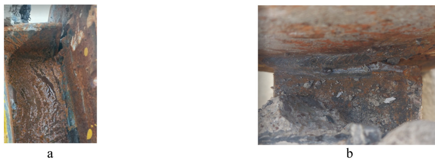
Figure 17: Shape of failure in welding of beam of CM4. (a) side view and (b) top view.
