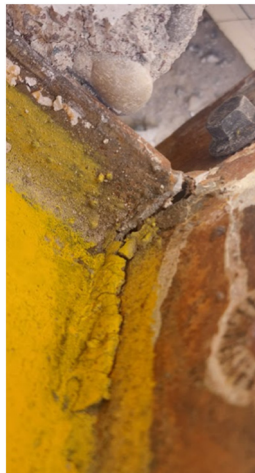
Figure 11: Shape of failure in welding of beam of CM2.
