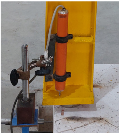
Figure 5: LVDT on a concrete slab.
