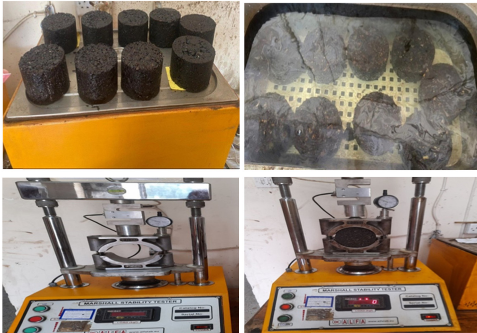
Figure 12: Marshall's device with test samples.
