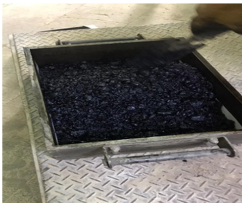
Figure 18: Paving of samples in the mold.
