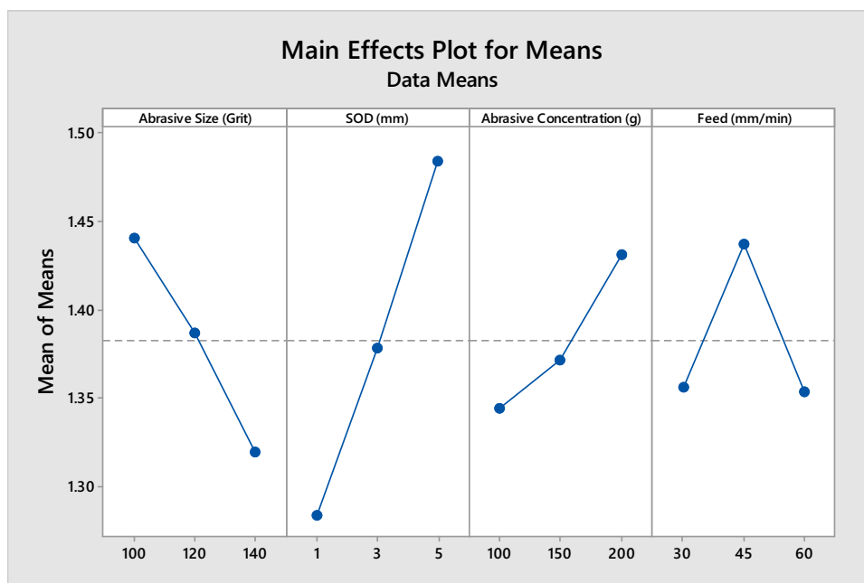
Figure 2: Main effects plot for means for MRR for free air cutting.
