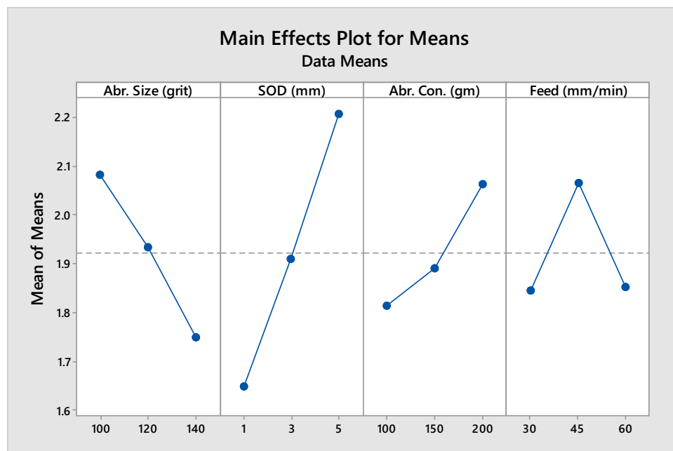
Figure 12: Mean of S/N for MRR for underwater cutting.
