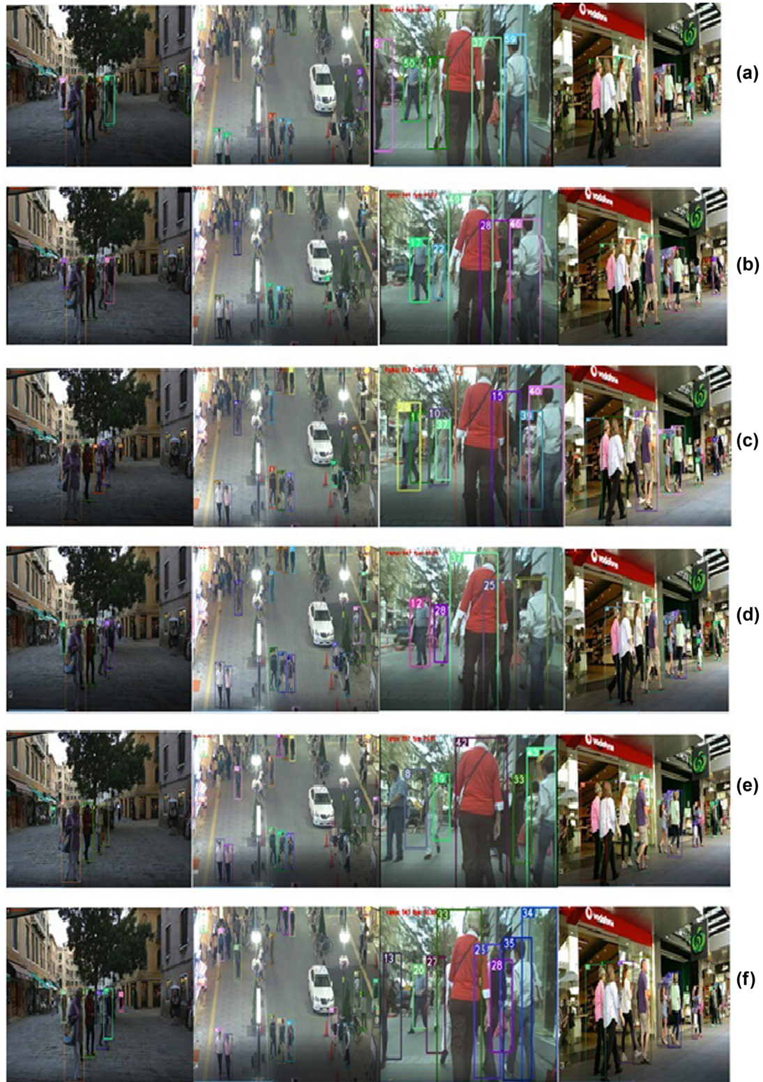
Figure 5: Videos output for different frame cancellation rates for normal mode and detector cancellation frame mode (a: Without cancellation, b, c, d, e, and f for 2, 4, 6, 8, and 9 frame cancellation rates, respectively) using Dataset MOT16: A Benchmark for Multi-Object Tracking [16].
