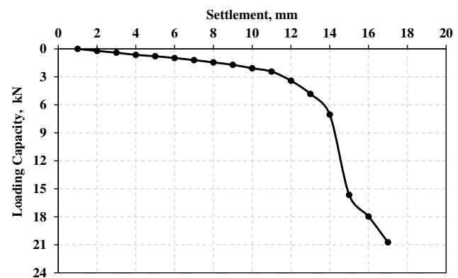
Figure 4: A typical load-settlement curve obtained from the plate loading test.
