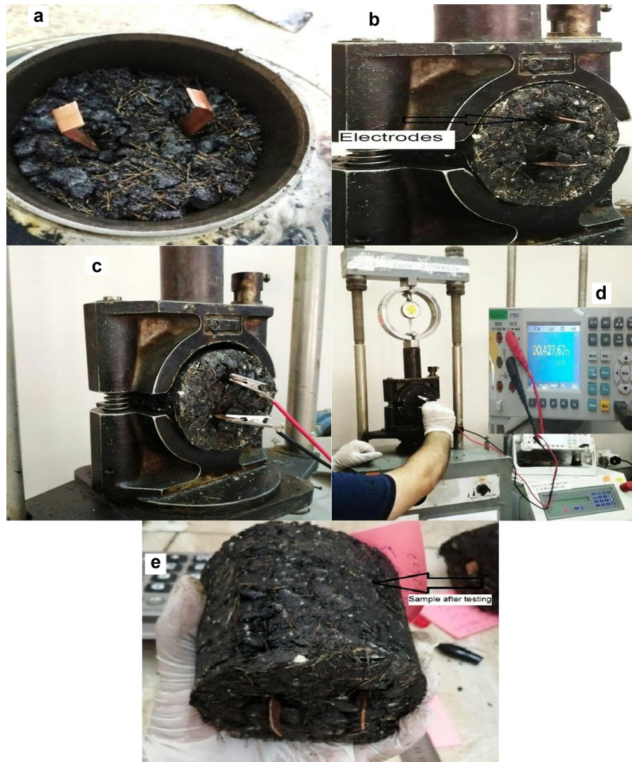
Figure 11: Stages of electrical resistivity measurement under Marshall test.
