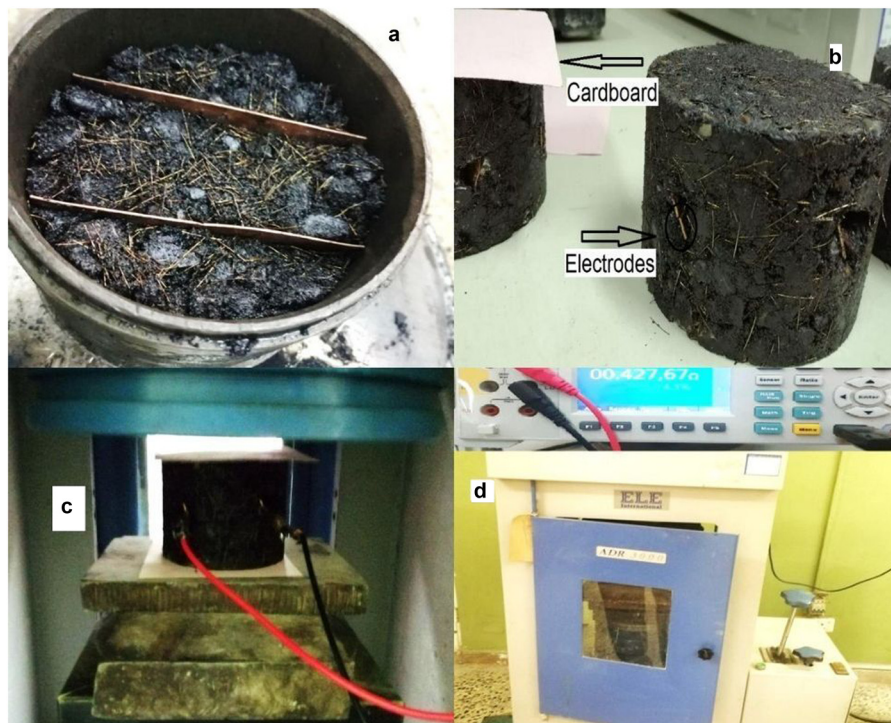
Figure 12: Stages of electrical resistivity measurement under compression test.
