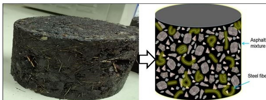
Figure 6: Detailed structure of HMA modified by SF.
