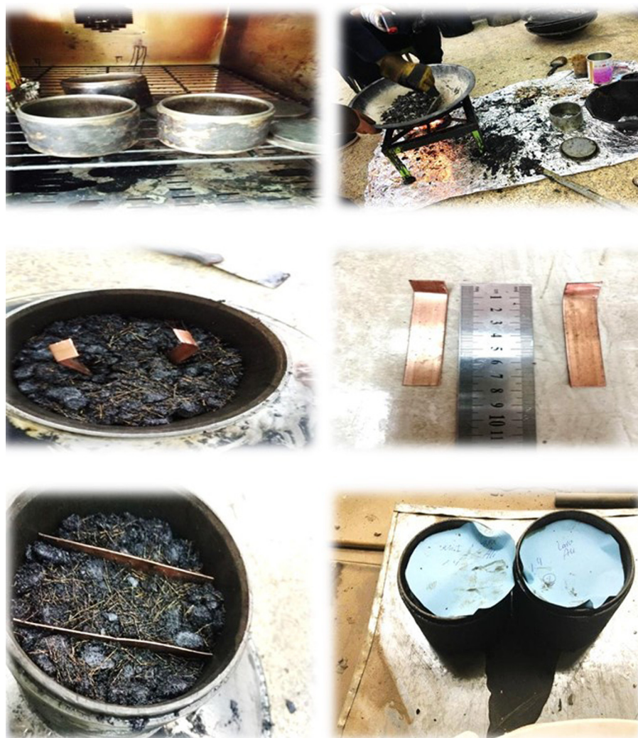
Figure 10: Stages of sample preparation and electrodes embedment.
