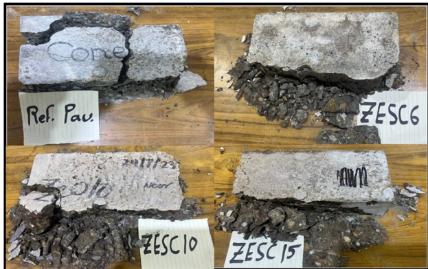
Figure 6: Compression crushed test specimen of reference ZESC paver mixes.
