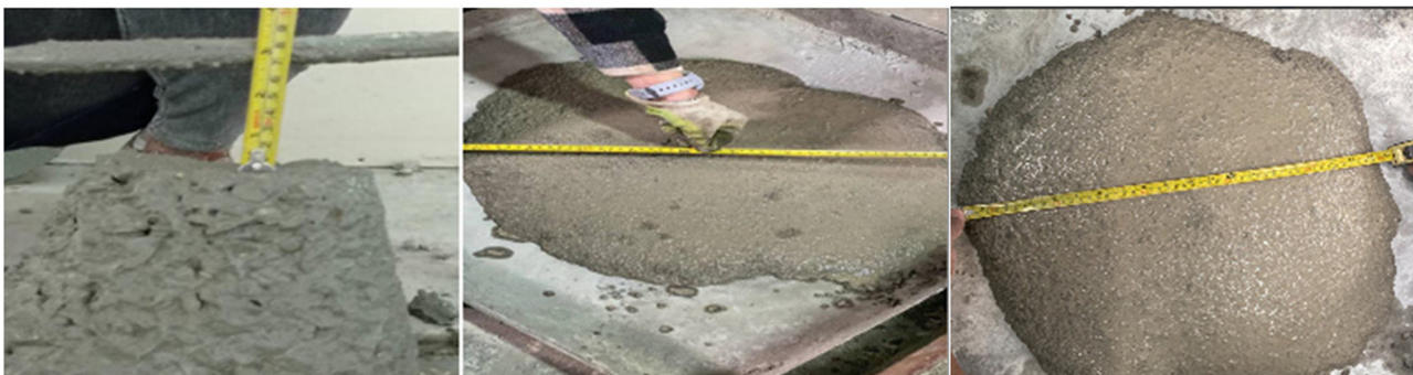
Figure 3: Value of slump test with or without adding superplasticizer to the concrete mixture.
