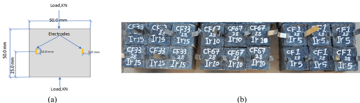
Figure 6: The geometric dimensions of the cubic specimens (a) and the manufactured specimens (b).
