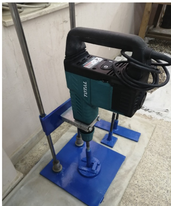
Figure 8: Vibration hammer for compacting RCC.
