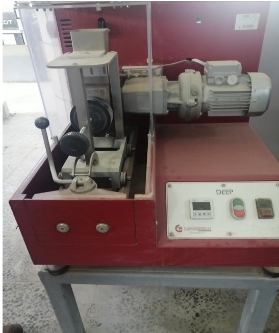
Figure 7: Abrasion test apparatus.
