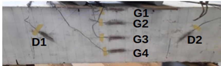
Figure 8: Location and names of strain gauges on concrete surface.
