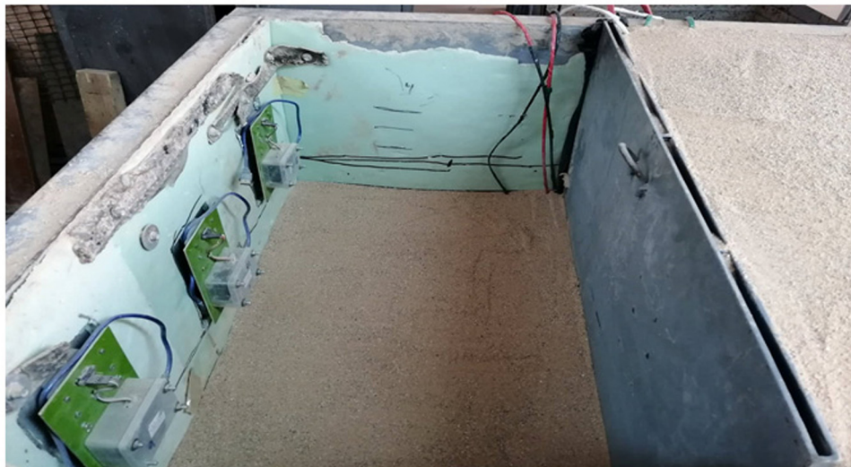
Figure 5: Placing the laser displacement in front of wall in the box.
