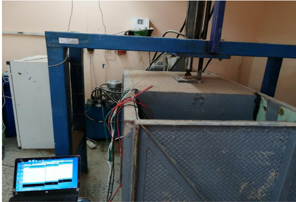
Figure 6: Model footing and retaining wall during the test.
