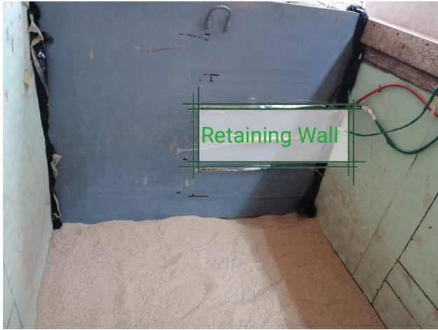
Figure 4: Manufactured retaining wall.
