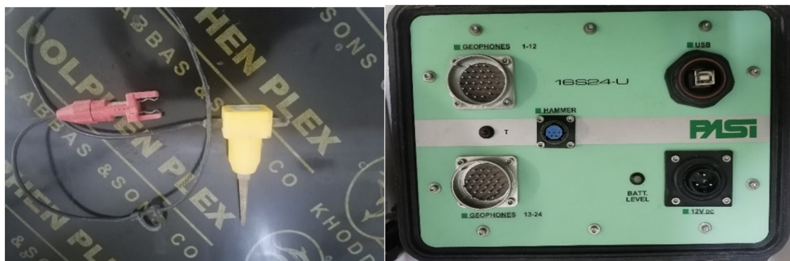
Figure 7: A 10 Hz geophone and Seismograph (PASI) data logger with 24 channels.
