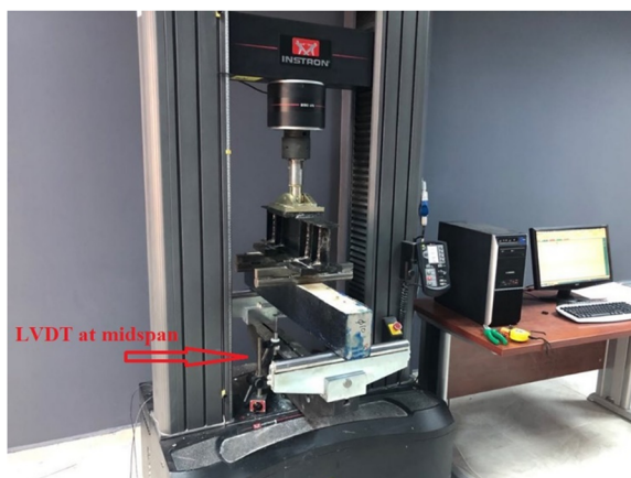
Figure 17: The flexure test setup.
