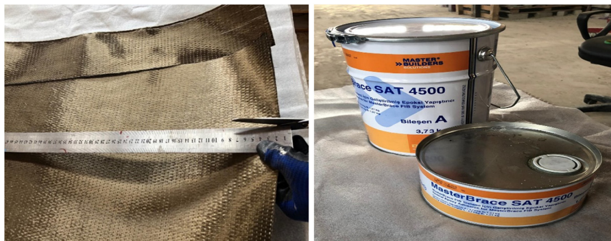
Figure 5: Epoxy resin used for bonding and BFRP sheets.
