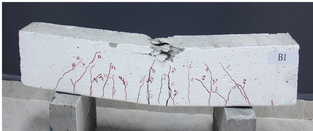
Figure 19: Crack pattern for beam B1.
