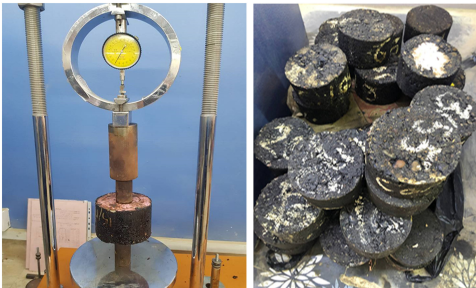
Figure 13: Samples under the double punch shear test.
