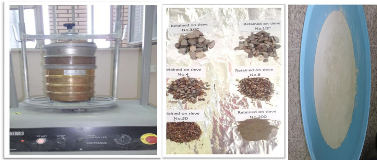
Figure 1: Sieve Shaker device and sieving sample.
