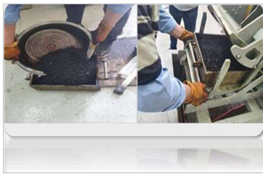
Figure 5: Slab specimens preparation by a roller compactor device.
