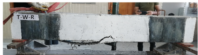
Figure 10: Beam with CFRP composites at the bottom and the ends.
