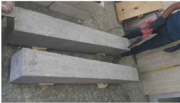
Figure 5: Surface preparation for the tested beams.
