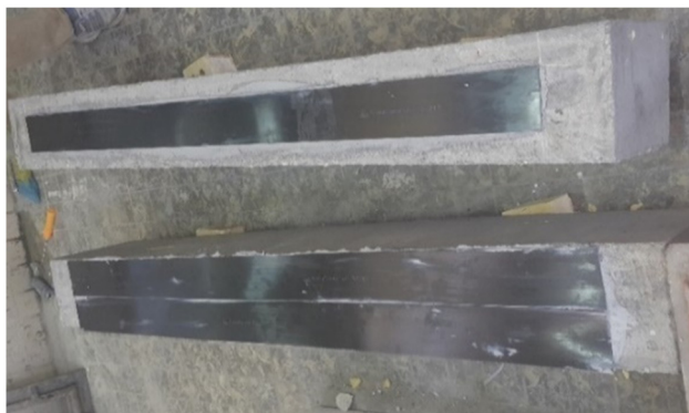
Figure 9: Beam with CFRP plates for group D.
