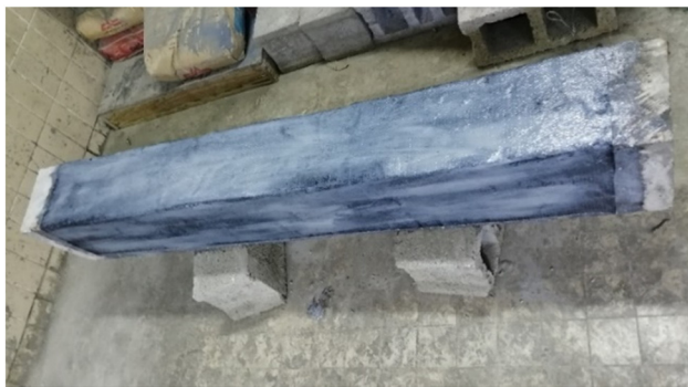
Figure 8: Beam with U-shape of CFRP woven.
