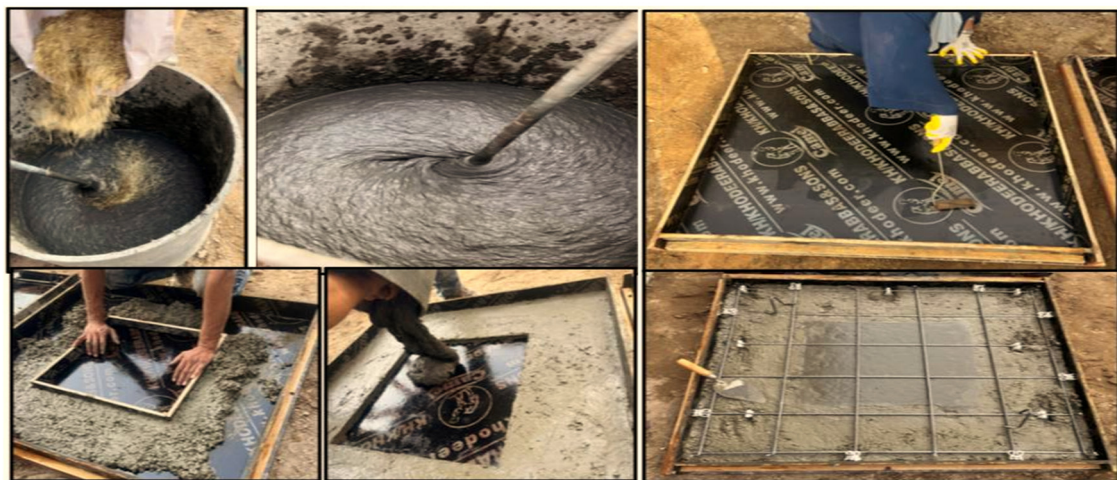
Figure 2: Cast slab with SIFCON layer.
