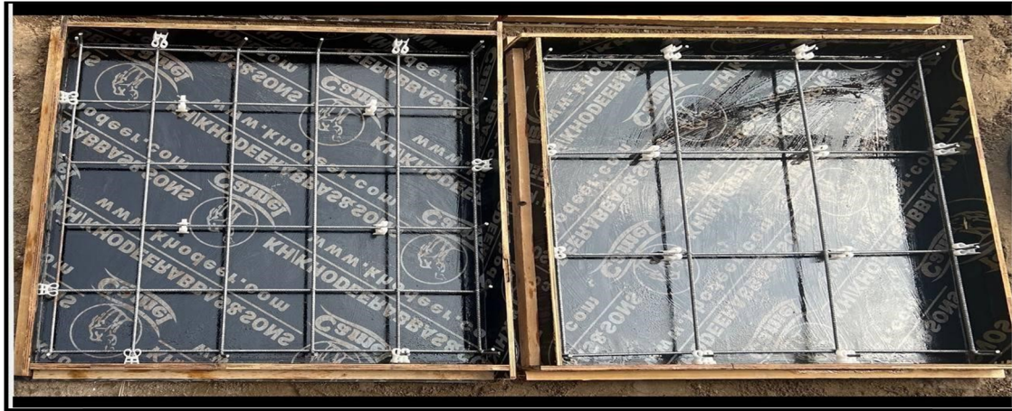
Figure 1: Flexural reinforcement of slab.
