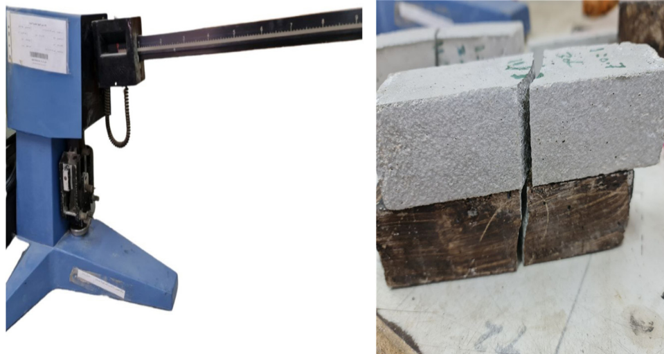
Figure 5: Flexural strength test.
