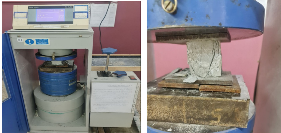
Figure 3: Compressive strength test.
