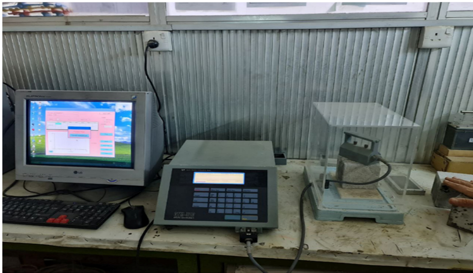
Figure 7: Thermal conductivity measuring apparatus.
