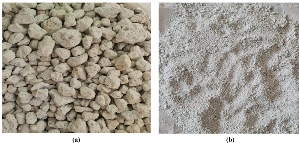
Figure 1: Lightweight Ponza aggregate: (a) before crushing and (b) after crushing.
