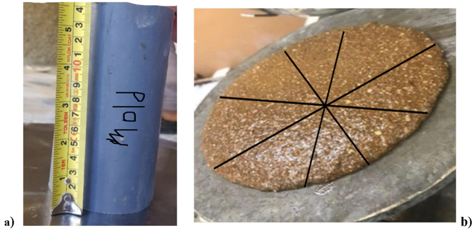
Figure 2: (a) Cylinder test. (b) Flowable mixture.
