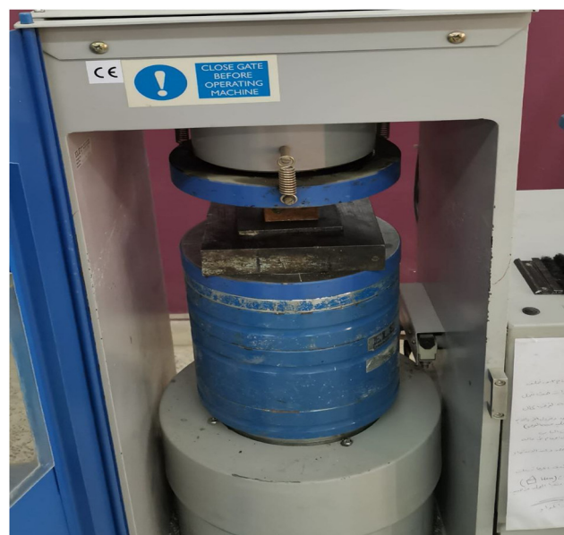
Figure 5: Compressive strength testing process.
