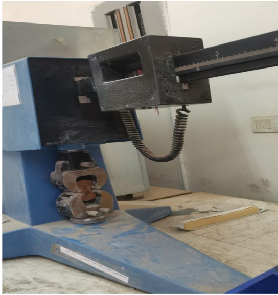
Figure 9: Direct tensile strength testing process.
