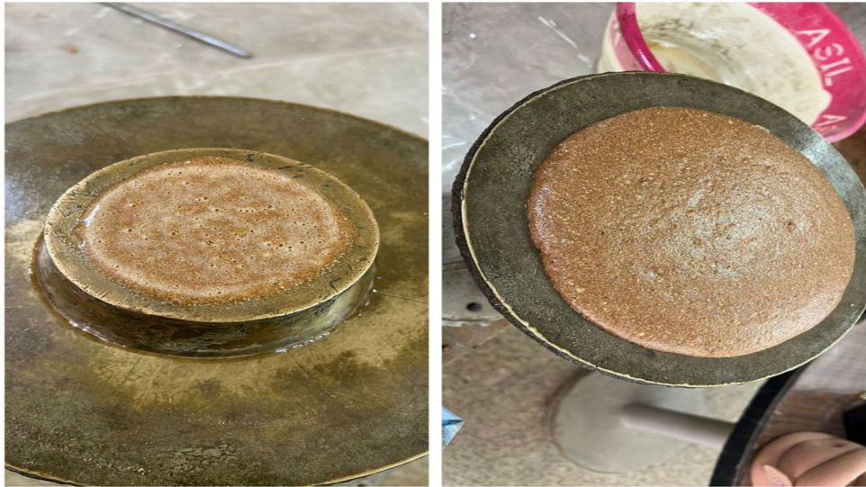
Figure 3: Flow-table testing process.
