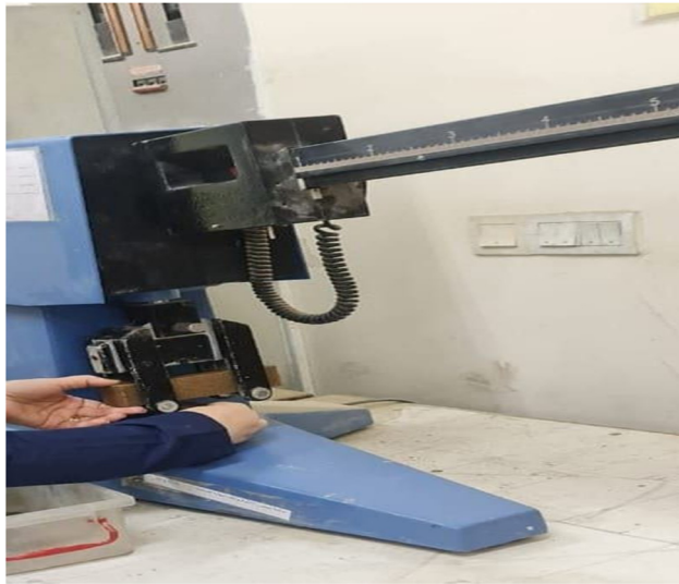
Figure 7: Flexural strength testing process.
