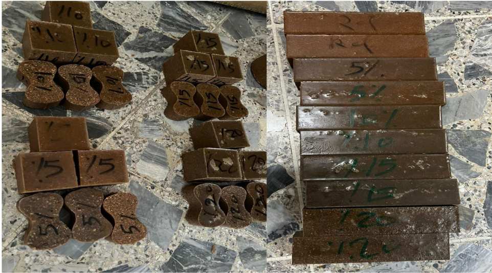
Figure 2: De-molding and curing of polymer mortar specimens.
