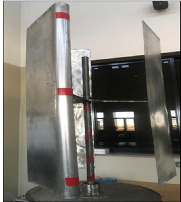
Figure 2: VAWT prototype with 1 m three-blade H-Darrieus.
