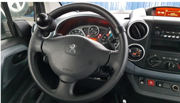
Figure 2: Handle in the form of a knob. Source: ITS.
