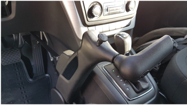
Figure 1: Pull-push device with accelerator lever. Source: ITS.
