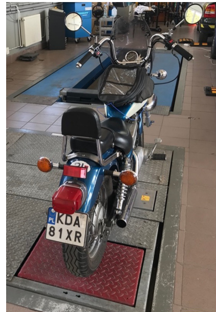
Figure 4: The motorcycle before the suspension test on the Bosch Beissbarth diagnostic line.
