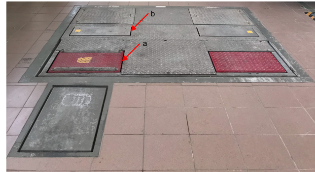
Figure 2: Beissbarth diagnostic line: (a) THETA SAT690 device and (b) EUSAMA SA640 device.
