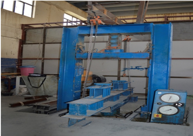
Figure 8: Universal testing machine and sample under one-point load.
