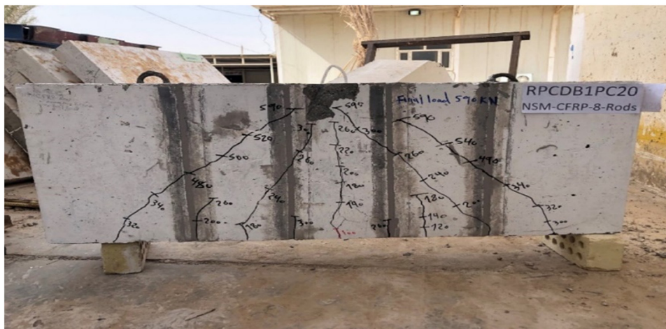
Figure 21: Crack pattern and failure mode RPCDB1P-8NSM.
