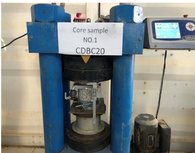
Figure 10: Testing compression machine with two gauges to calculate the strains.
