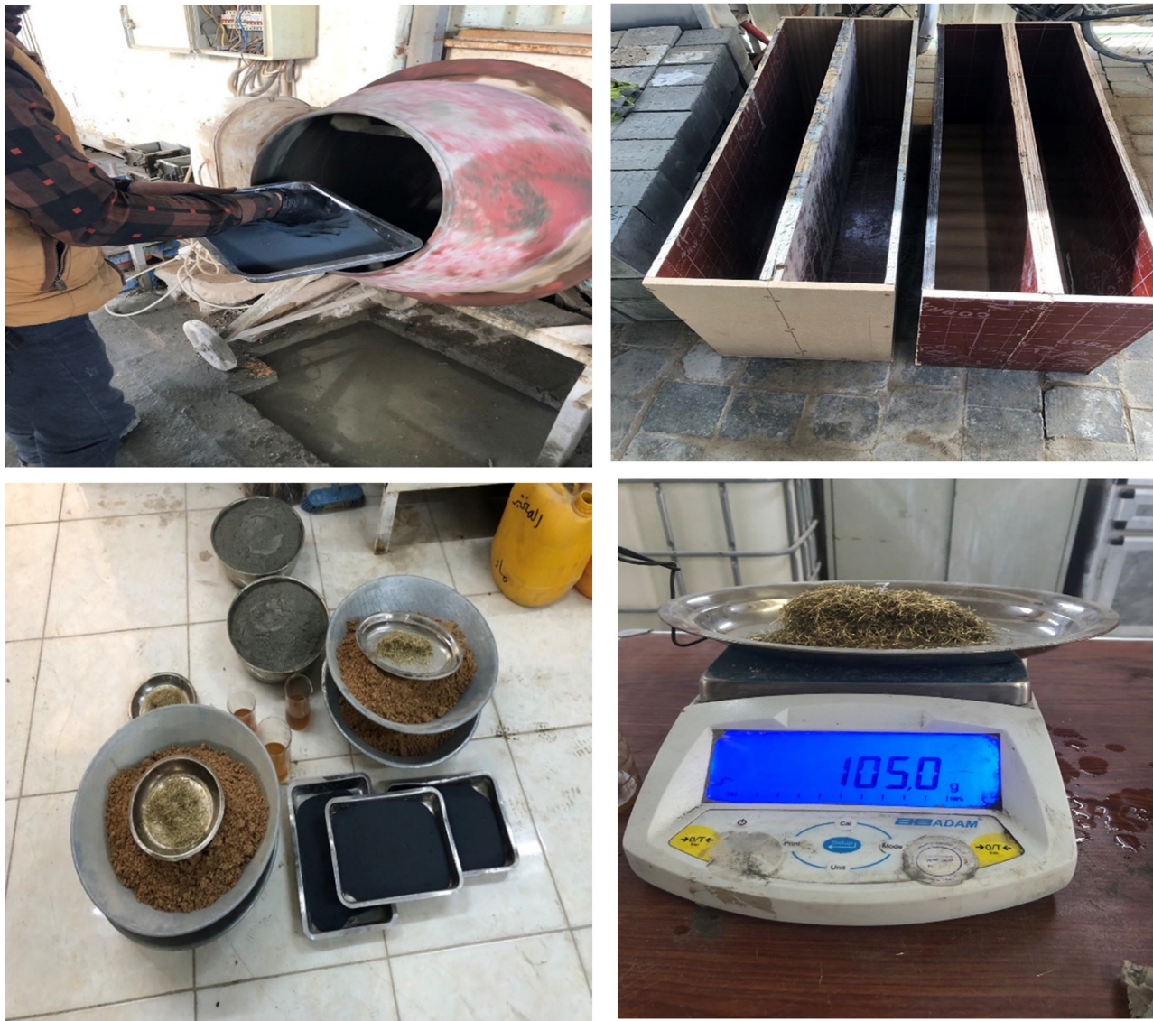
Figure 2: Specimens' preparation and materials of RPC.
