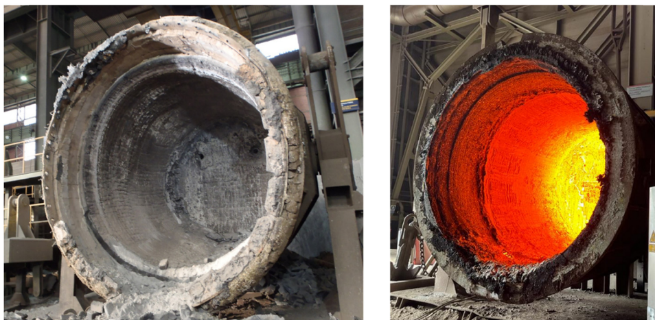
Figure 5: Left: Used steel ladle taken out for demolition of lining. Right: Hot steel ladle, after visual inspection and waiting for next heat.
