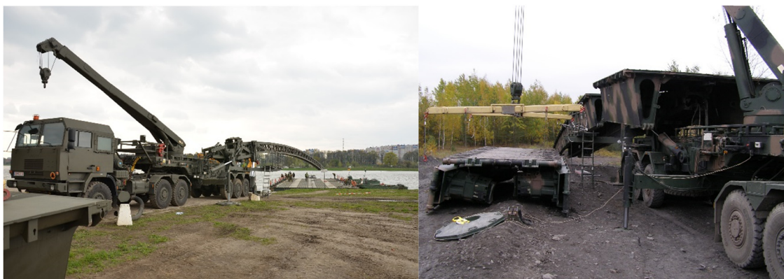
Figure 4: A vehicle with an MS-40 launching system.
