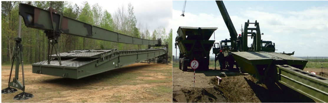
Figure 5: Different types of launching beams, DSB (on the left) and MMK (on the right) [2].
