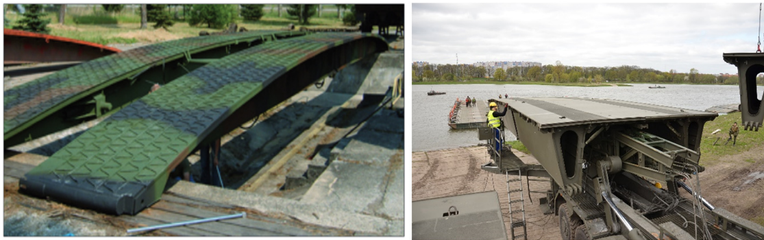
Figure 2: Types of spans: the BLG-67 [11] with treadways on the left and the MS-40 span with no gaps between treadways.
