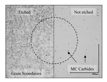
Figure 7: Estimated indentation size with respect to the elements of material structure.
