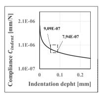
**Figure 18:** Estimated changes (using equation (16)) in compliance  $C_{indent}$  with respect to the indentation depth for ball indenter with 2.5 mm diameter made from tungsten carbides.
