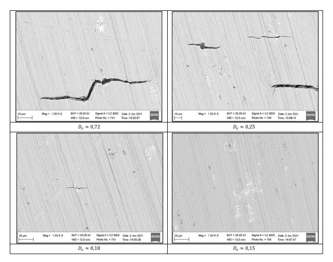
Figure 11: Surface of the gage part – HCF.
