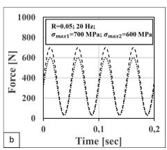
Figure 3: Load scheme for mechanical test performed on speciemns used for the investigation. Tensile test (a) and fatigue test (b).
