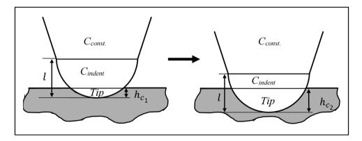
Figure 17: Illustration of machine frame contact stiffness components.
