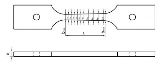
Figure 2: Specimen with varying cross-sections of the gage part used for the investigation.
