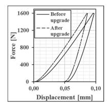
**Figure 20:** Force-displacement plot from indentation test before and after modification of displacement measuring system.
