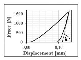
Figure 6: Force-displacement plot from indentation test.
