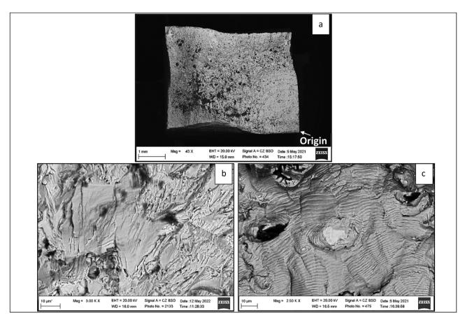
Figure 12: Fracture surface (a), origin area (b) and fatigue zone (c) of the specimen after LCF test.
