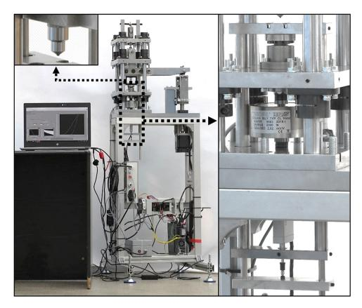
Figure 5: Device for instrumented indentation test.
