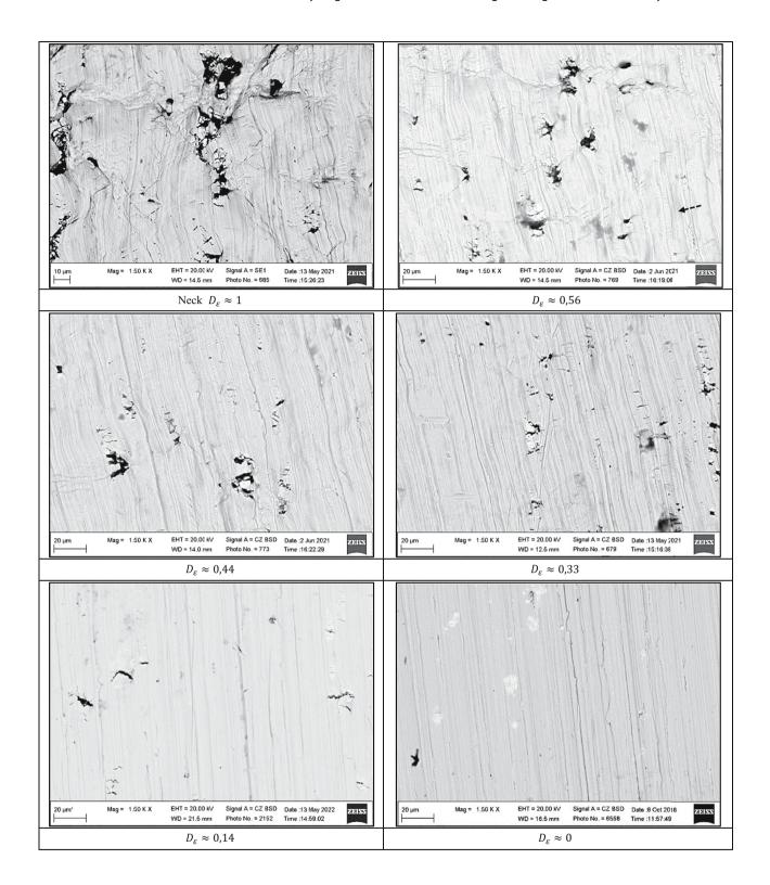
Figure 9: Surface of the gage part – static tension.
