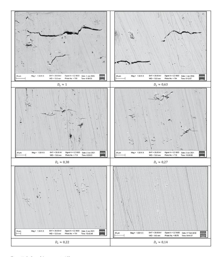
Figure 10: Surface of the gage part – LCF.
