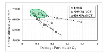
Figure 16: Results of contact stiffness measured for specimens after tensile test and fatigue test in areas with different values of damage parameter  $D_c$ .
