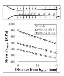
Figure 4: Stress distribution in specimen gage part.
