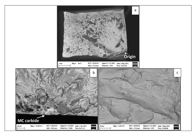
Figure 13: Fracture surface (a), origin area (b) and fatigue zone (c) of the specimen after HCF test.
