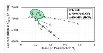
**Figure 19:** Results of contact stiffness measured for specimens after tensile test and fatigue test in areas with different values of damage parameter  $D_{\varepsilon}$ . As shown in Figure 16, green area correspond to early stage of damage developed in specimen after LCF test.
