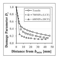
Figure 8: Distribution of the damage parameter in the gage part of the specimens after tests.
