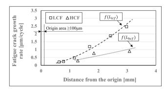
Figure 14: Chart representing the fatigue crack growth rate for specimens after LCF and HCF tests.
