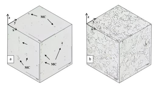
Figure 1: Image of the alloy used in the test. Before (a) and after (b) etching.
