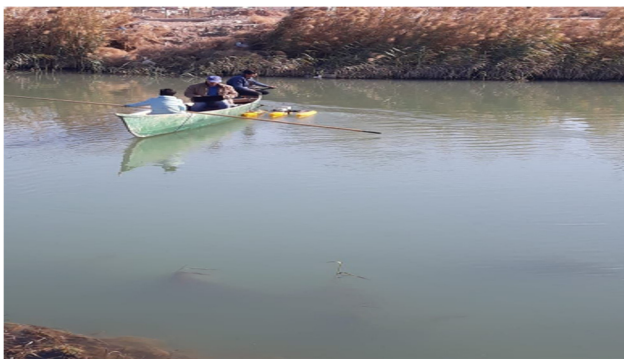
Figure 4: Measuring the discharge and velocity of each section along the channel using ADCP.
