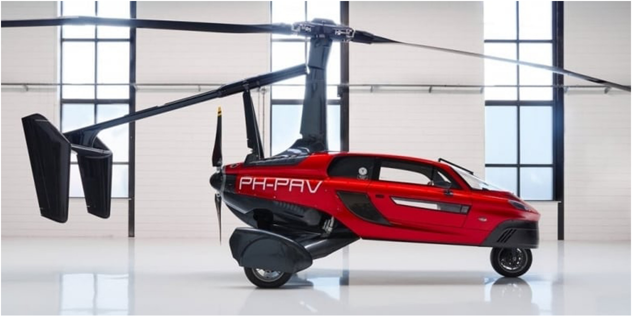
Figure 6: PAL-V Liberty Sport from outside with extended rotor and propeller (image credit: PAL-V International B.V., used with permission).
