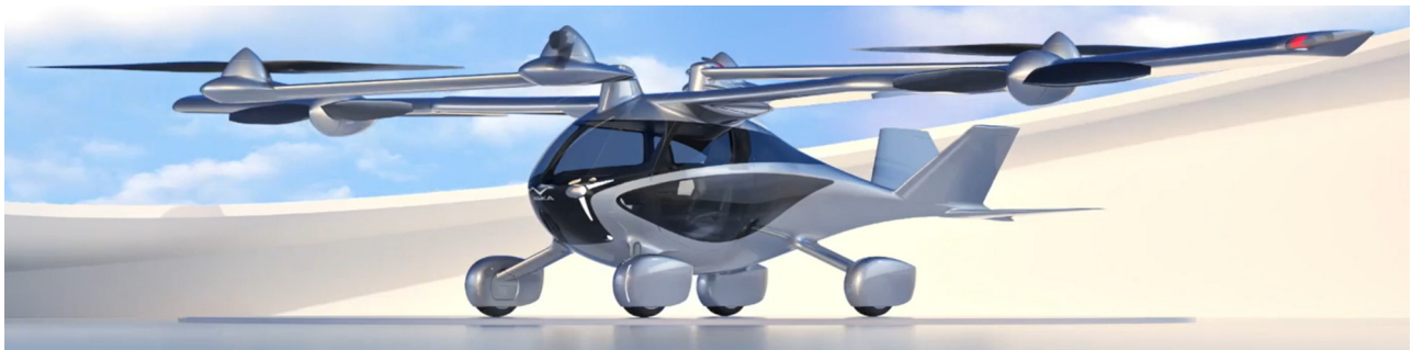
Figure 9: An imagined view of the ASKA flying car with the wing and propeller-carrying arms extended (image credit: NFT Inc., used with permission).
