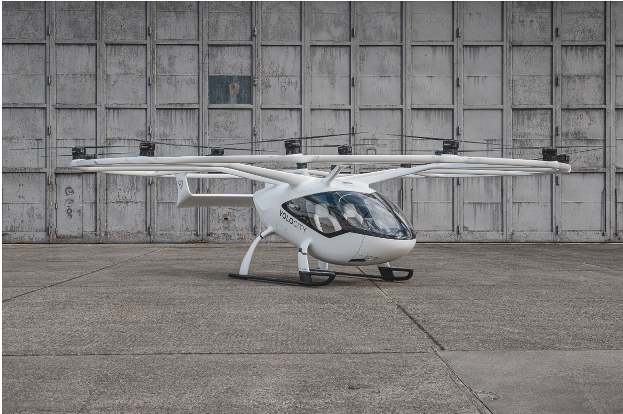
Figure 3: A real model of Volocopter’s VoloCity air taxi, aimed for commercial UAM services (image credit: Volocopter GmbH, used with permission).
