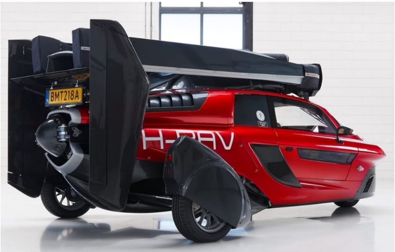
Figure 7: PAL-V Liberty Sport from outside with folded rotor and propeller (image credit: PAL-V International B.V., used with permission).
