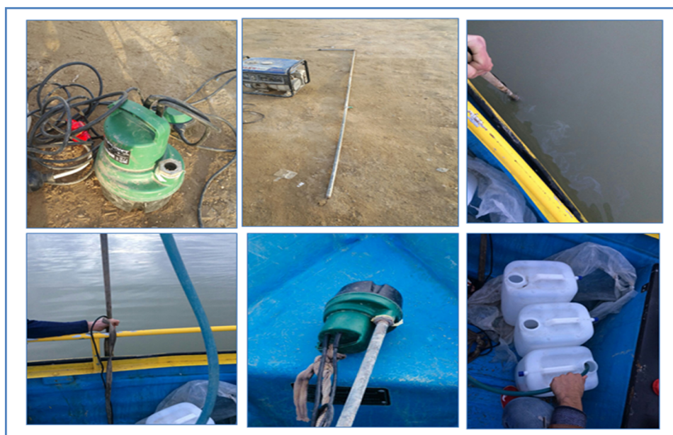
Figure 1: The method of withdrawing samples of water at various depths.
