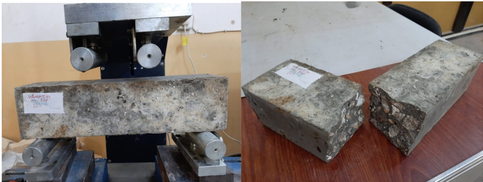
Figure 3: Flexural strength test for 100% waste tile concrete – modified mix.
