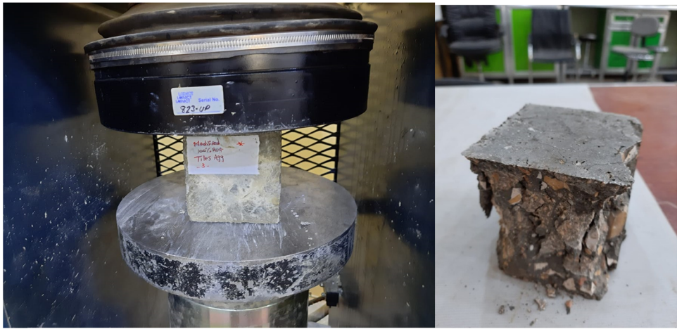
Figure 2: Compressive strength for 100% waste tile concrete – modified mix.
