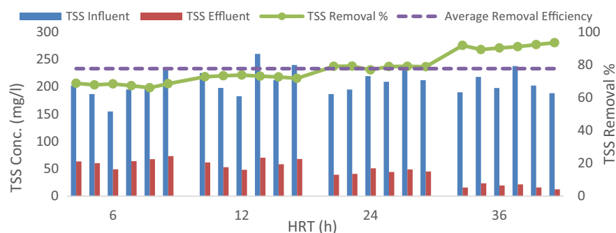
Figure 4: Average TSS removal during steady-state conditions at various HRTs of 36, 24, 12, and 6 h.
