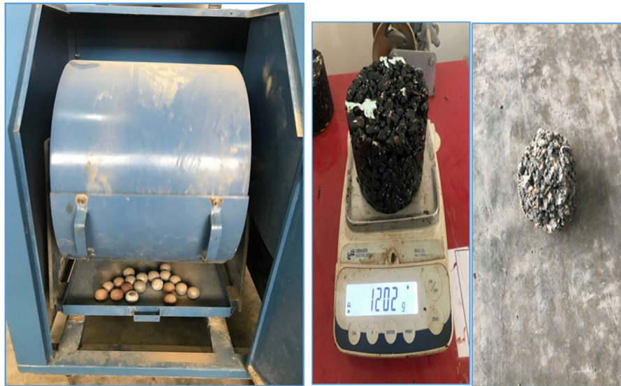
Figure 2: Los Angeles abrasion test.
