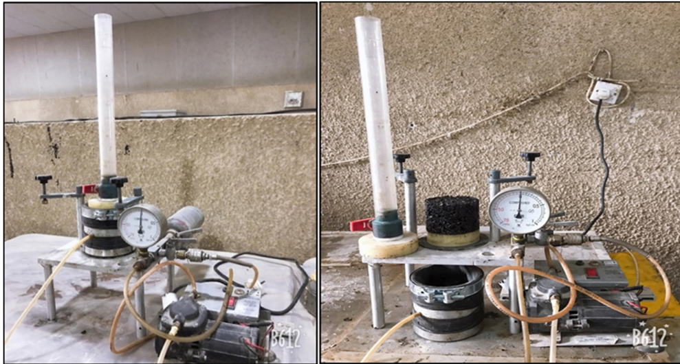
Figure 4: Hydraulic conductivity apparatus.
