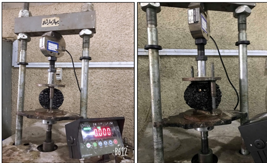
Figure 5: The indirect tensile test by Marshall device.
