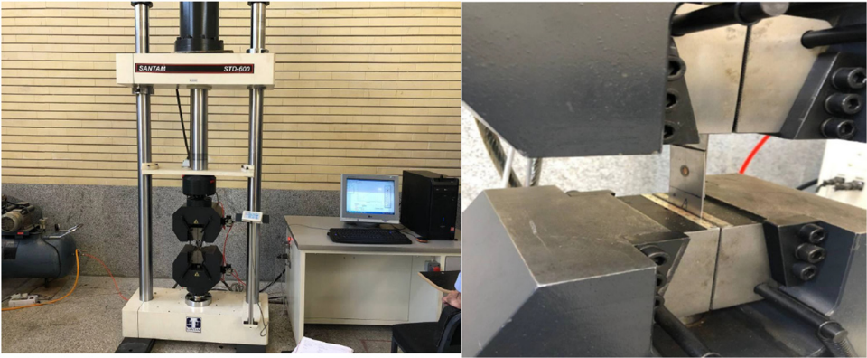
Figure 10: Tensile shear test.
