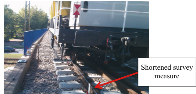
Figure 4: Geodesic measurements of rail deflections under a ballast-carrying wagon.
