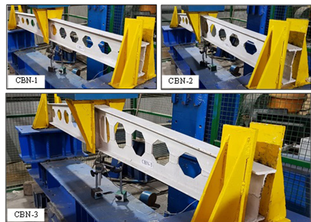
Figure 12: Test setup of TCBs (CBN-1, CBN-2 and CBN-3).
