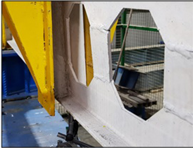
Figure 13: Failure mode of TCB (web post buckling).
