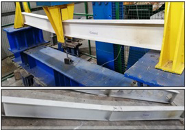
Figure 7: Failure mode of control specimen.
