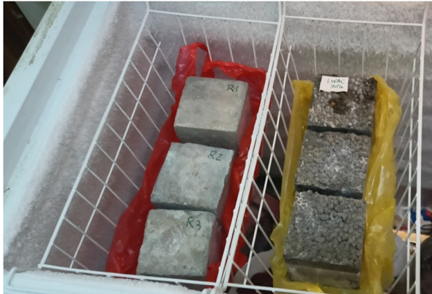
Figure 5: Specimens under testing for FTCs.
