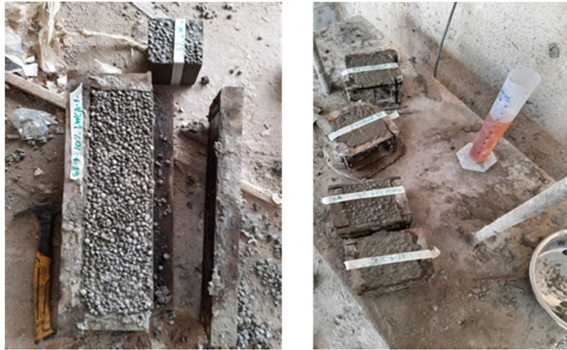
Figure 3: Some cubic concrete specimens with 3% replacement after casting and concrete beam with 10% replacement during mold open.
