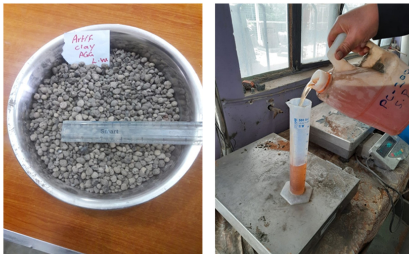
Figure 2: Artificial expanded clay and PC-200 superplasticizer.
