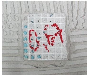
Most cohesive separation inside of adhesive, average force 0.67 kN
