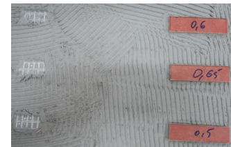
Most cohesive separation inside of adhesive
