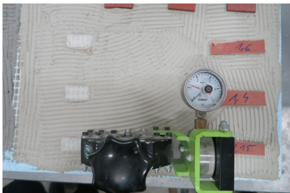
Figure 4: PressoMess for shear strength testing
