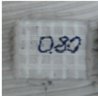
Cohesive separation inside of adhesive, average force 0.74 kN
