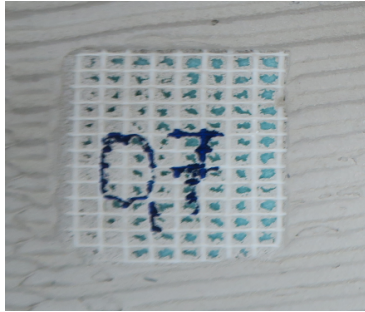
Adhesive separation from XPS, average force 0.70 kN
