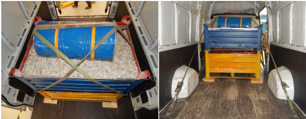
Figure 3: Securing of the 1000 kg load with high COG. Source: Authors
