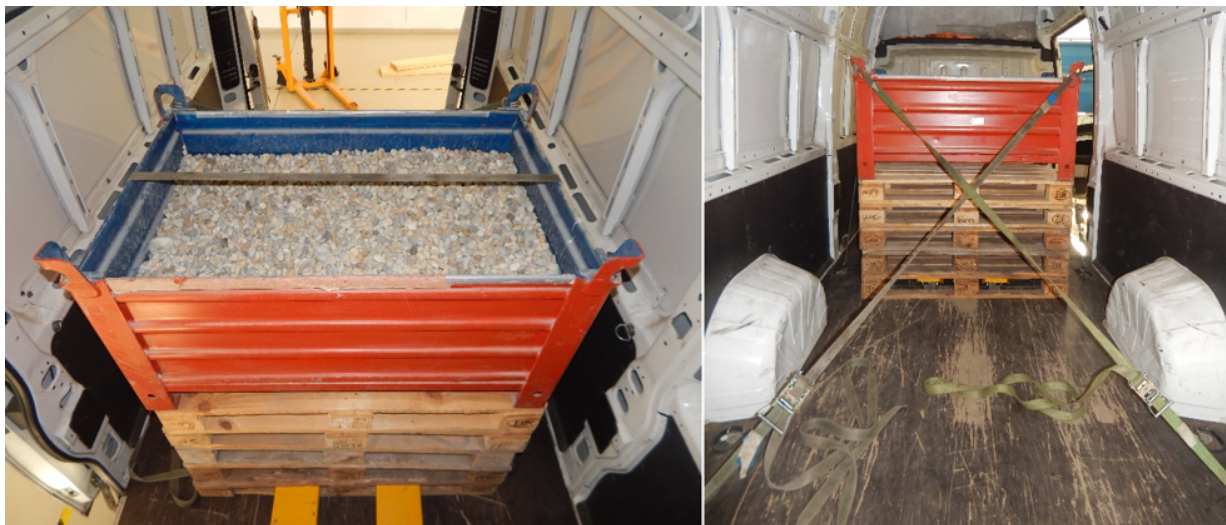
Figure 4: Securing of the 500 kg load with high COG. Source: Authors
