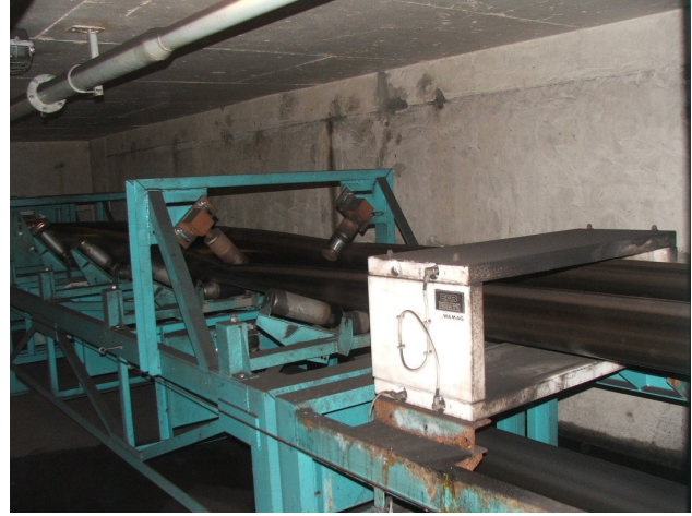
Figure 3: Electromagnetic device for removing metallic particles [8]
