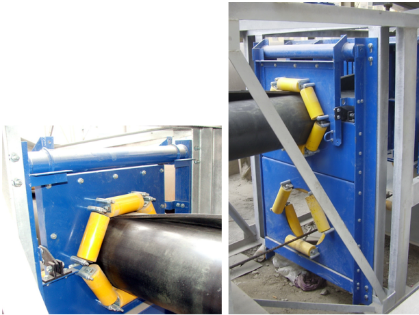
Figure 2: Material flow monitor with horizontal opening [8]
