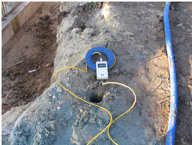
Figure 12: A view of BAT test execution in DSM wall.
