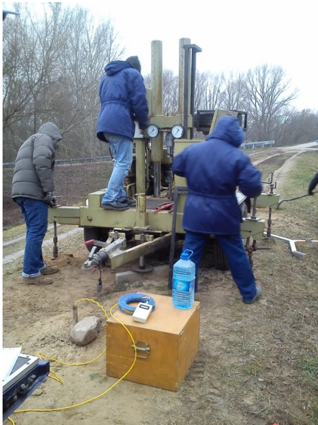
Figure 6: A view of CPT and BAT test execution.
