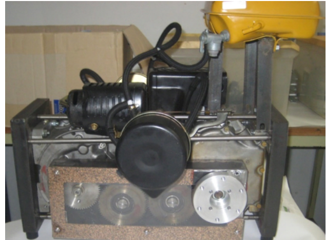
Figure 4: Final positioning of the reciprocating piston engine PTO for this design.
