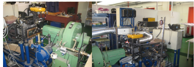
Figure 5: Overview of the dynamometric test bench and the opposing piston engine.
