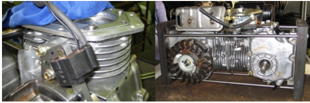
Figure 3: Detail of aluminum spacer, engine head gasket and union guides.
