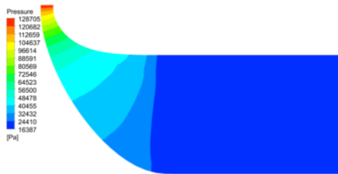
Figure 12: Static pressure in the rotor averaged along the circumference.
