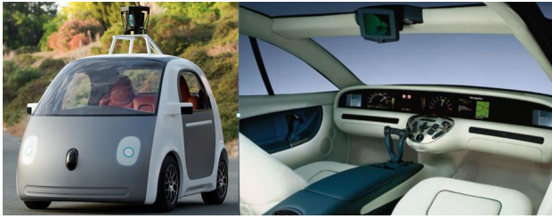
Figure 9: Google's two-seater self-driving car prototype eliminates steering wheel, accelerator and brake pedals.
