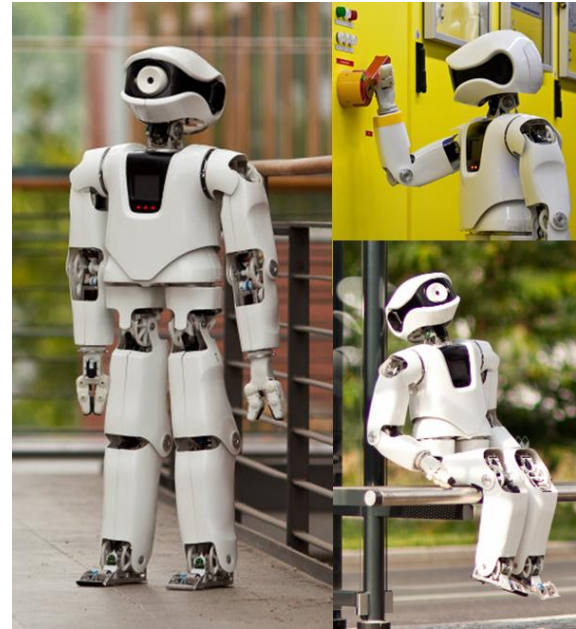
Figure 7: Myon the child-like cognitive robot developed by the Neuro Robotics group at Humboldt university.
