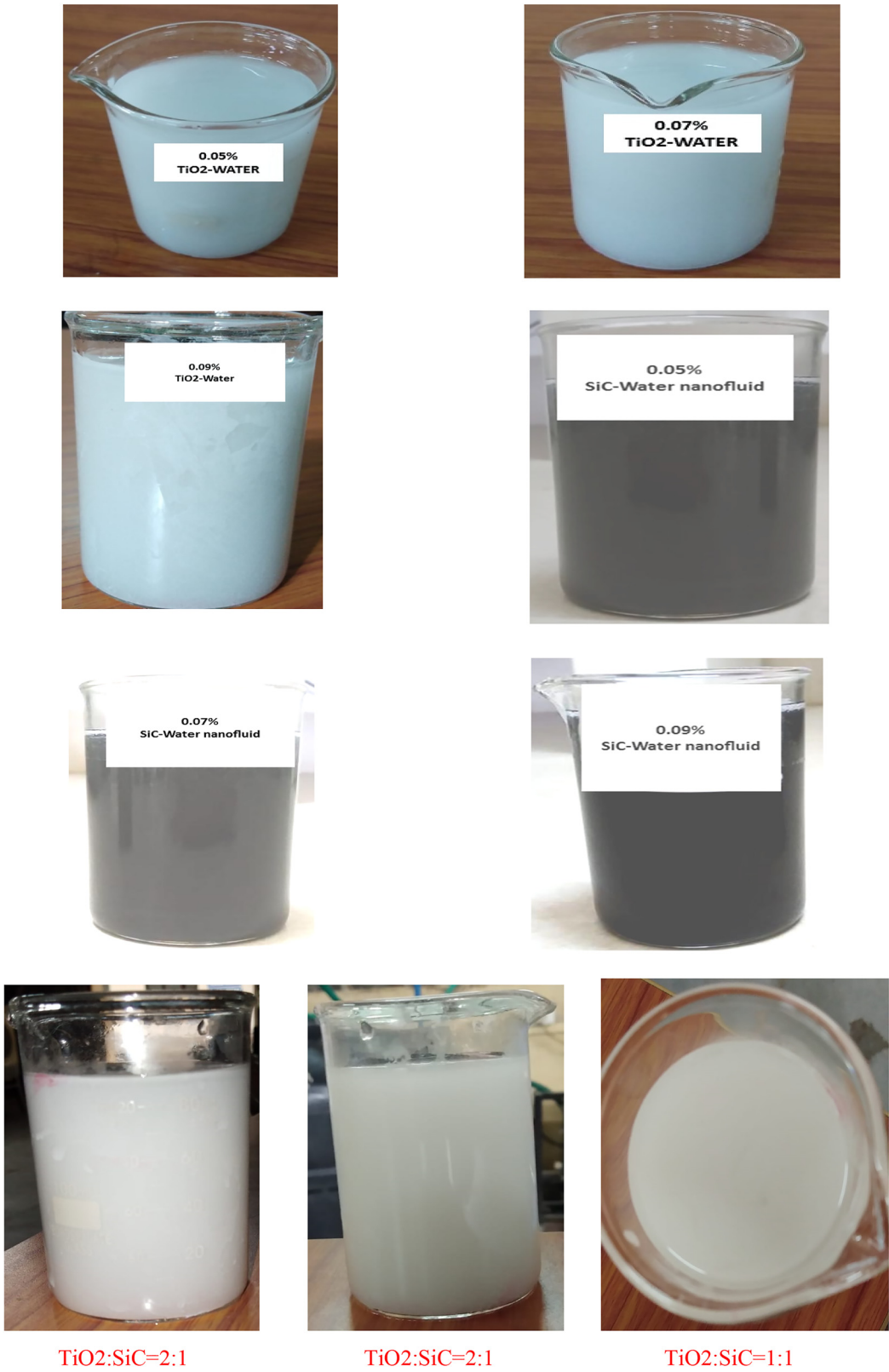
Figure 6: Nanofluid samples with different percentage volume concentrations.
