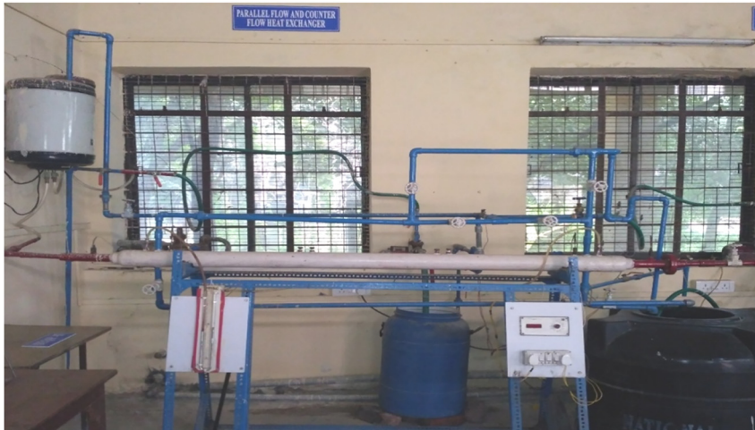
Figure 2: Experimental setup of double pipe HE.
